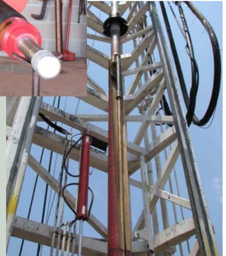
Weatherford's IPP inflatable packer provides a positive, pressure-tight seal for annular isolation between the work string and casing or open hole to assist in remediation or abandonment applications during drilling, production, or intervention.
