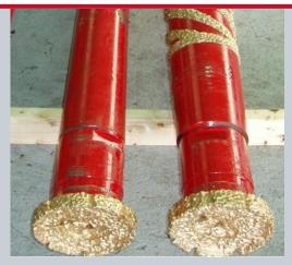
The *MillThru* system's square-shouldered mills provided the technology to engage and mill through the lateral liner and back into the main bore of the well.
