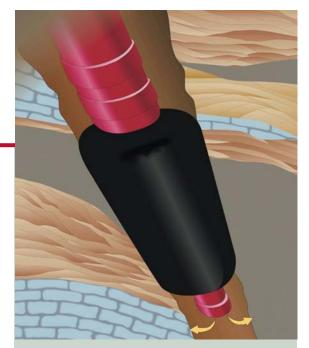
Weatherford's *IPP* packer provides a positive, pressure-tight seal for annular isolation between the workstring and casing or open hole to assist in remedial or abandonment applications during drilling and production. Compatible with drillpipe, threaded tubing, and coiled tubing, this packer offers the versatility of a temporary or permanent seal for single- or multiple-packer configurations in wells of any deviation.
