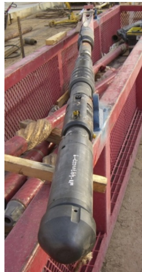
The Weatherford retrievable whipstock assembly (center) includes an ISO V3-rated retrievable packer for isolation and a 3° concave for deflecting the QuickCut milling assembly through the casing wall.
