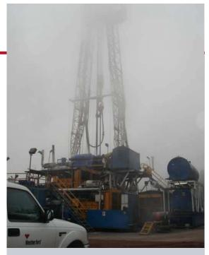
A Weatherford openhole screw-in whipstock successfully sidetracked this Mexican geothermal well. High temperatures made a conventional sidetrack with a cement plug impractical.
