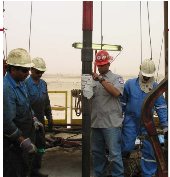
Crew members deploy the re-entry deflector assembly.
