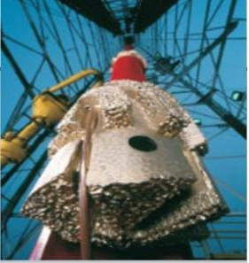
Weatherford's shallow-angle *QuickCut* casing exit whipstock system's single-trip design and the high-expansion *MultiCatch* casing exit system anchor provided the operator with unmatched flexibility, creating an exit window and saving rig time and associated costs.
