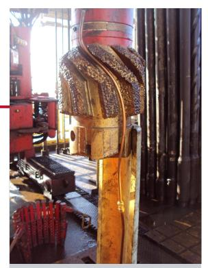
The shallow-angle *QuickCut* casing exit whipstock system's single-trip design and the high-expansion *MultiCatch* casing exit system anchor provided unmatched operational flexibility. This combination created an exit window through multiple casing strings, saving rig time and associated costs.
