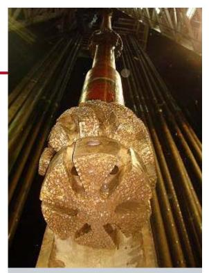
Weatherford's shallow-angle *QuickCut* casing exit system with hydraulically actuated *MultiCatch* anchor provides the milling, gaugeretention, and formation-drilling performance in a single trip that mature-field applications require.
