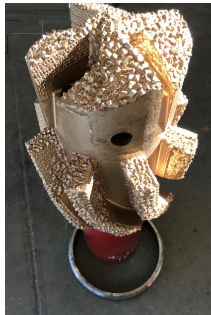
The lead mill is gauged before it is attached to the BHA.
