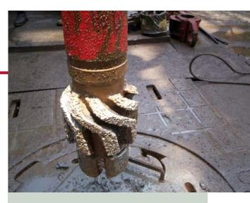
The ShallowAngle *QuickCut* casing exit system, with *CustomCut* tungsten carbide inserts, cut through Q125 high-yield casing in one trip, proving its capabilities to Shell and another major operator for a high-profile job in the North Sea.
