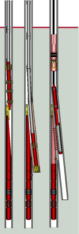
The *StarBurst* multilateral system, with a hollow whipstock, creates a longer window exit, using minimal weight. This capability helps avoid pipe buckling and other problems in ultra-deep well applications. The system provides a Level 4 junction with full-liner access to the lateral bore.
