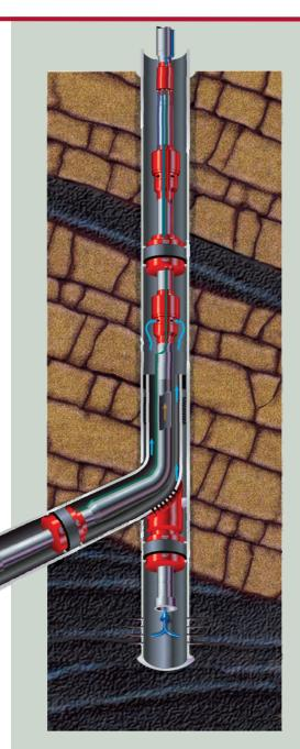
The *StarBurst* hollow-whipstock multilateral system is ideal for wells in mature fields where production rates are declining and additional nearby reserves can be drilled and produced while maintaining production from the original wellbore.
