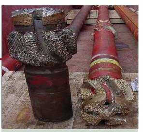
Using the shallow-angle *QuickCut* system allowed the operator to create a window exit and rat hole in a single trip with negligible gauge loss.
