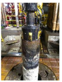
The Weatherford DHPT facilitates application of extreme forces downhole directly into any type of stuck fish, such as casing, drill pipe, tubing, drilling BHAs, packers, and plugs. The system enhances safety and operations efficiency by running the tool downhole, thereby eliminating all tensile forces off the workstring and rig surface equipment.
