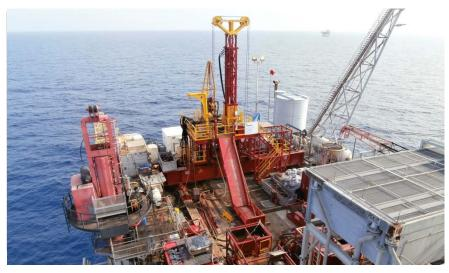
The Weatherford Rig-Free 35/1000 light-duty pulling and jacking unit has a pulling capacity of 35,000 lb (15,876 kg) and a jacking capacity of 1,000,000 lb (453,592 kg).
