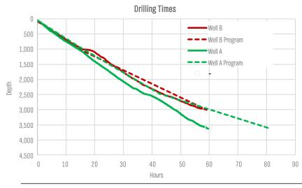
The above graph illustrates drilling times in Well A (green) and Well B (red). Although the drilling program estimated 82 hours of drilling time in Well A, the actual time took 60 hours, which equates to 22 hours saved.
