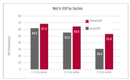
Before operations began in Well A, the drilling program established estimates for rate of penetration (ROP) according to past performance. The above graph shows that the actual ROPs exceeded the planned ROPs in each section.
