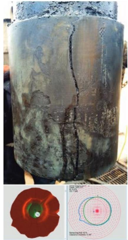
The Weatherford SecureView service provided an exact casing-hole evaluation for a leaking well in the Wolfcamp shale formation. The pulled casing (top) shows damage identical to the damage indicated by the logs (bottom).
