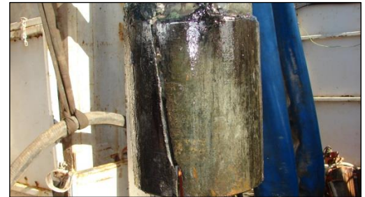
Physical examination of the pulled casing verified the analysis of data from the Weatherford SecureView suite and revealed the casing collar split shown above.
