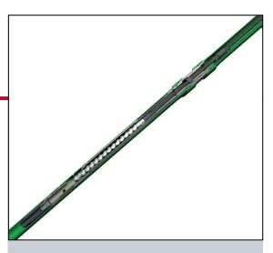
Weatherford's patented *Arrowhead* I-PCP design reduces the length of the assembly during running and pulling. The pump eliminates the need for production tubing to be pulled and re-run during servicing operations because the rod string is used to install or remove the I-PCP from the well, reducing operational time and cost.
