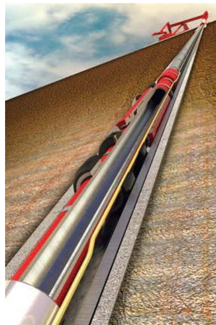
The Weatherford capillary-injection tubing anchor has a bypass channel that enables the capillary string to reach the pump inlet for targeted chemical delivery.
