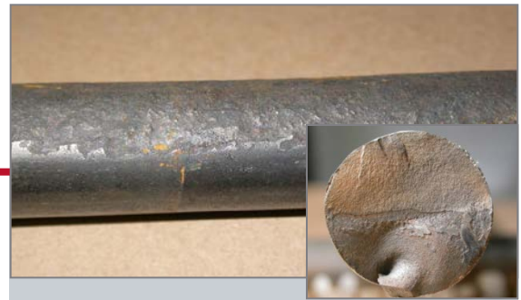
Sample of continuous rod that failed from corrosion fatigue after 3 months.
