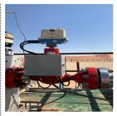
The Weatherford EAMV utilizes a field-proven, intermittent vent-controller with a three-way pilot valve classified as a non-bleed device for cleaner operations.
