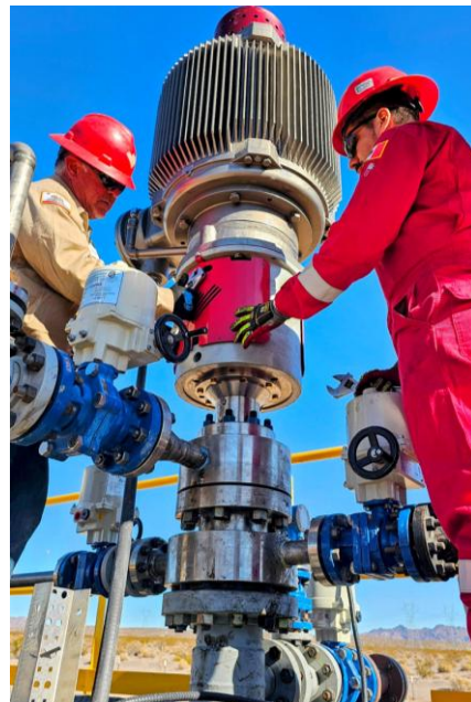
Ready for borate production, the modified I-PCP with PMM is installed at the 5E Advanced Materials location in Newberry Springs, California.
