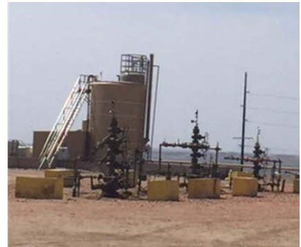
Gas lift is designed for maximum production in sandy conditions and deviated wellbores.
