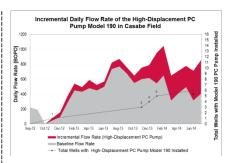
Incremental daily flow rate increased in the six wells with the Weatherford high-displacement PCP model 190
