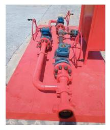
With no moving parts, the Weatherford surface jet pump delivers a cost effective, rigless production enhancement for a variety of applications including natural-well augmentation and wellhead backpressure reduction. For wells with naturally declining production rates, the surface jet pump will boost production levels without a workover unit and only minor modifications to pump components.
