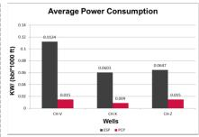
Average power consumption comparison of ESP and PCP artificial-lift systems installed on three wells of the field.
