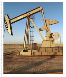
The Weatherford Permanent Magnet Motor (PMM) demonstrated its energy-saving value over diesel-driven wells at Shahd field in Egypt. The PMM is an AC-synchronous, direct-drive system that provides high-torque/low-speed power that is up to 98% efficient. By eliminating all belts and transmission drives, PMMs boost production performance while reducing emissions and improving overall safety with virtually maintenance-free production.
