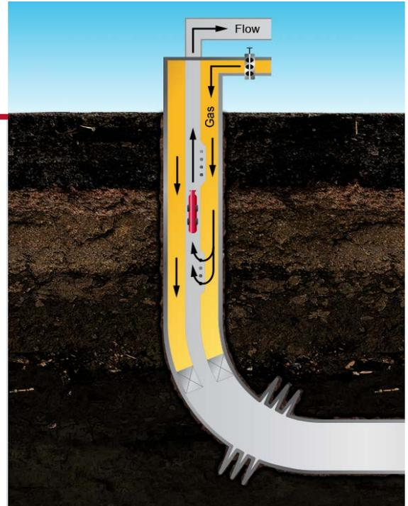
The unique bypass valve in Weatherford's *RapidFlo* plunger enabled the operator to maximize flow time and avoid paraffin cutting.
