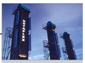
Weatherford's unique-designed Rotaflex long stroke pumping units feature a stroke length of up to 25.5 ft (7.8 m) and an innovative 100%-mechanical reversing-mechanism design.
