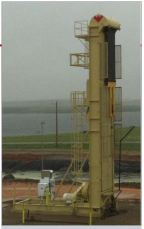
The Rotaflex long-stroke pumping unit increased oil production in historically costly, high water-cut environments.
