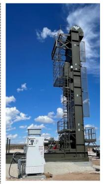
The Weatherford Rotaflex long stroke pumping unit combined with ForeSite Power regenerative system VSD and the PMM direct drive creates next generation energy efficiencies from all three technologies, providing higher levels of production performance and cost saving value.
