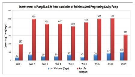
After the installation of stainless steel PCPs in nine wells, pump run life significantly improved while workovers decreased, despite corrosive downhole conditions and the completion of several acid stimulations.
