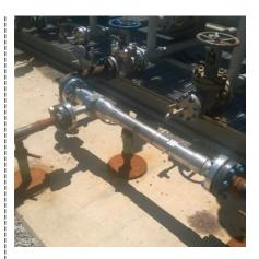
With no moving parts, the Weatherford surface jet pump delivers cost-effective, rigless production enhancement for a variety of applications including natural-well augmentation, and wellhead backpressure reduction. In a well with naturally declining production rates, the surface jet pump will boost production levels without a workover unit and only minor modifications to pump components.
