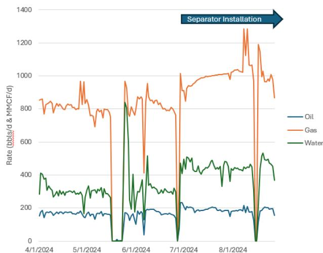
Post-workover installation of TOPS improved gas release, eliminated ESP overheating, and increased production by 27%.
