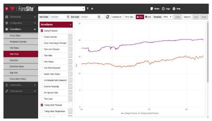
An image from the ForeSite software platform: Monitoring casing pressure (purple) and tubing head pressure (orange) and optimizing production through surfactant dosing rate.
