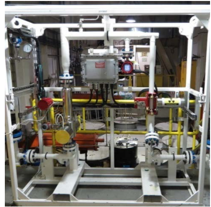
The Weatherford Alpha VSRD was installed on a platform in Cook Inlet Alaska to provide allocation measurement.
