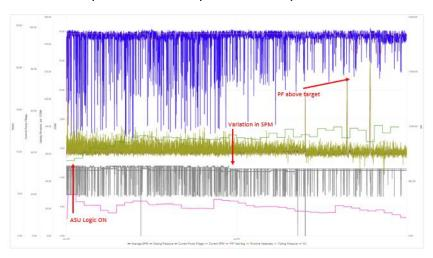
Autonomous control based on speed change met to stabilize the well and optimize production
