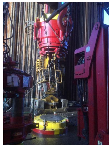
Multi-pipe size catch range for each slip set reduces slip change requirements especially for tapered strings.
