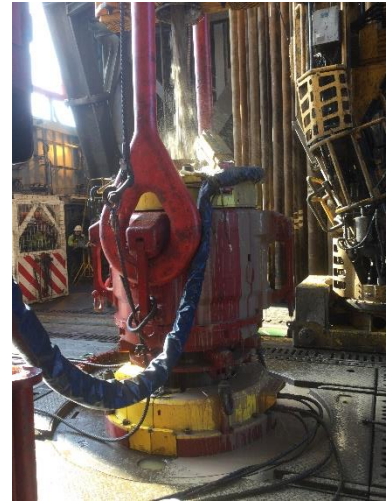
Multi-sized slips and elevator provides running solutions for loads up to 1,500 tons (1,360,777 kg) of drillstring, casing, and tubing.
