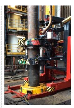
Based on the thread-specific parameters, the onboard computer monitors and controls the makeup sequence for the system. It continually monitors several process outputs and proactively adjusts the inputs to achieve a consistent final makeup precisely to the desired parameters.
