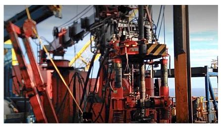
The Vero system replaces human judgment and influence with computer-controlled consistency and accuracy during makeup, completing the entire connection makeup and evaluation process using an onboard computer, sensors, and programming.
