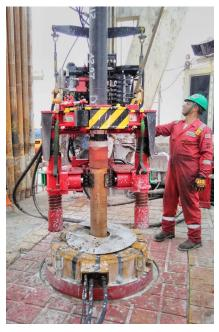
With a single push of a button, a Weatherford team member initiates the final makeup process.
