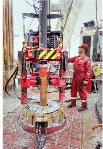
Operated with a simple push of a button, the Vero conventional system controls the makeup and evaluation of premium pipe connections on land and shallow-water rigs.
