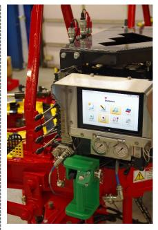
When put to the test, the Vero system successfully detected a damaged joint during the spin-in process for completion tubing. It also replaced the ESP for the completion with zero rejected joints.
