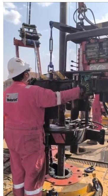
The Vero conventional system, RCS-500 completions slips, and the AutoCLAMP system.
