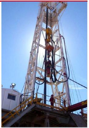
The remotely operated *OverDrive* system enhanced crew safety by eliminating manual handling of tubulars, reducing the number of personnel required on the rig floor while enabling remote users with specific expertise the ability to monitor well progress in real time.
