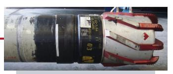
The 20- x 24-in. *Defyer* DPA 8419 casing bit was used to drill the 20-in. casing string through a 1,802-ft (549-m) interval—the longest, deepest section that Weatherford has drilled to date with a 20-in. *DwC* casing-drilling system.
