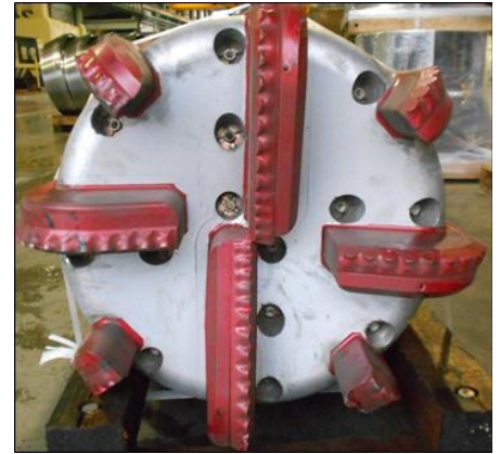
Using a 20 × 24-in. Defyer® DPA8419X casing bit, Weatherford drilled a 387.74-m (1,272.11 ft) interval with 20-in. casing string in one run.
