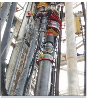
Weatherford's *OverDrive* casing running and drilling system, with the *TorkDrive* tool, greatly enhances safety by combining the functions of power tongs, elevator, fill-up circulation tool, weight compensator, and bails. This technology provides faster tubular makeup and breakout without thread damage. It minimizes risk by reducing the crew requirement and eliminating the need for a stabber.
