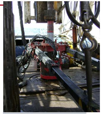
The OverDrive system allows the driller to rotate and push (or pull) the casing string while circulating, making it ideal for high-angle, extended-reach wells. It overcomes drag on long strings of lateral pipe, mitigates wellbore sloughing, and efficiently handles other instability issues.
