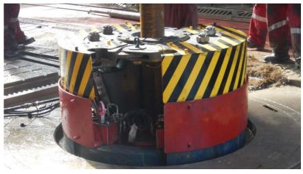
The LSS 1250 acts as a spider to safely and efficiently grip tubulars, and has a load capacity of up to 1,250 tons (1,133,981 kg).
